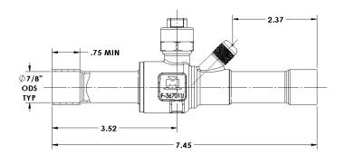
CYCLEMASTER® Ball Valves are UL/cUL Listed, conform to the Pressure Equipment Directive 2014/68/EU.
