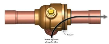
When viewed from the top, if the stem arrow points away from the tubes, refrigerant flows to the side opposite the weld joint.
