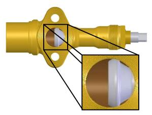
Always thoroughly wetwrap valve before brazing, confirming that stem packing and body cavity are protected.
