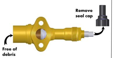
2 Ensure stem is in mid-seat (half-open) or back-seat (fully-open) position before applying heat. Valve *MUST NOT* be closed (front-seated) during brazing operation.
