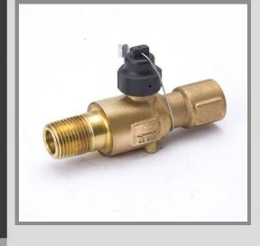
Ball isolation valves for relief valves (BIR) are designed to ensure that there is no flow restriction created during normal operation with the attached relief valve or rupture disc assembly, while providing complete isolation of the circuit when necessary for routine maintenance or replacement.
